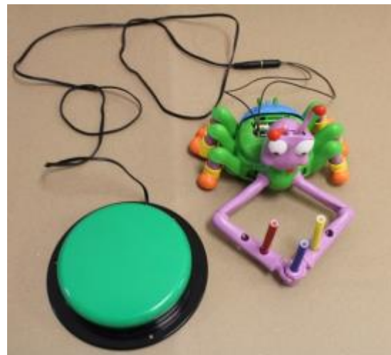
Doodle Doug scribbling device adapted with a battery interrupter so it can be controlled with a switch. The student may need assistance with the cord as it may get tangled when Doug spins.
